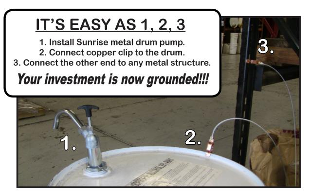
Don't forget to buy your metal drum pump, copper clips and grounding wire when you purchase products in a drum! **Protect your investment and prevent static discharge!**
